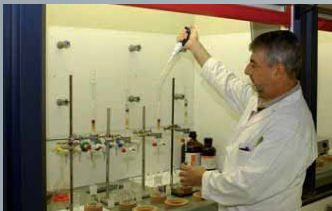
▲ Sample preparation (clean-up) for the analysis of PCBs : Hugo Franken (2004).
