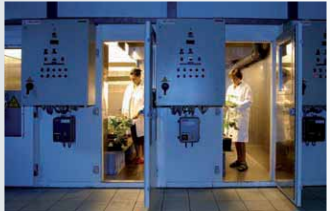
▲ Climatic chambers for ozone exposure of test plants : Annick Evrard (left) and Karine Vandermeiren (right) (2004).
