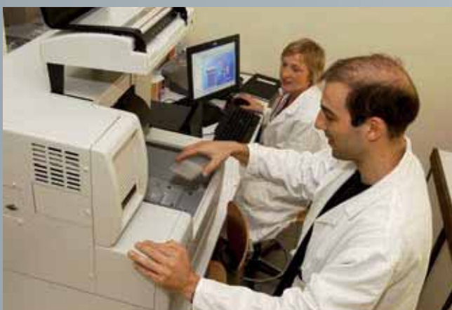
▲ Preparation of a sequence reaction using a Beckman CEQ8000 Genetic Analysis System : T. Stakenborg and A. Pil (2004)
