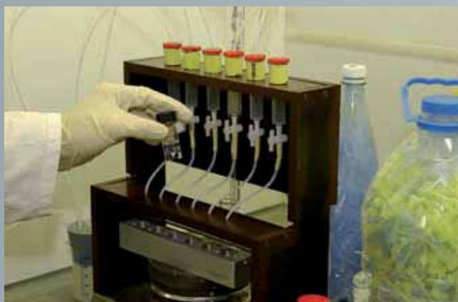
▲ Sample preparation (derivatization) for the analysis of T2/HT2 toxins (2004).
