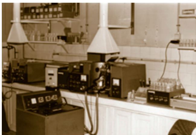
▲ Atomic absorption spectrometry equipment for heavy metal analysis (1976)
